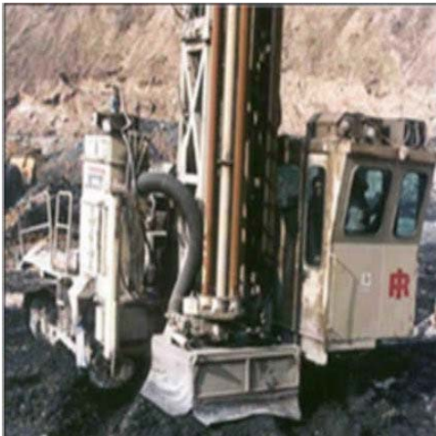
Vehicle-mounted drilling rigs with dust collection system around drill bit and low-flow water spray to wet the dust discharged from the dust collector. The enclosed operator's cab is on the right. The dust collection system is on the left.
